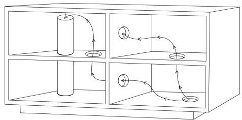
the floor itself so that you can create a "snorkel" running from just an inch or so below the top of the cabinet down into the lower level where it can be attached to the intake (suction) side of an Active Thermal Management Cool-cube®, ordered with 4" flex tubing.
